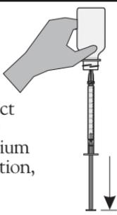
Fill another Direct Reading Titrator (0376) with Sodium Thiosulfate Solution, 0.025N (4169).
