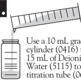
Use a 10 mL graduated cylinder (0416) to add 15 mL of Deionized Water (5115) to the titration tube (0608).
